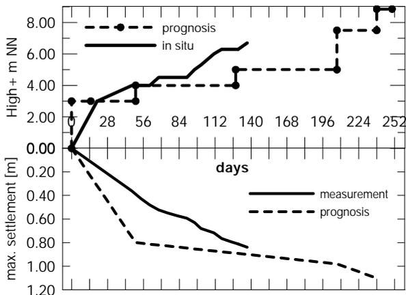
Figure 8: Measured settlements in section VI
