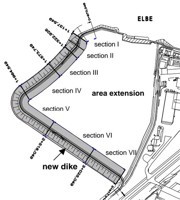
Figure 1. Concept to reclaim land by the construction of a polder
