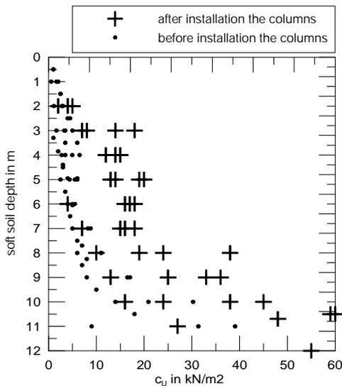
Figure 7. Increase of the undrained shear strength in the soft soil between the columns in comparison before and after installation the columns
