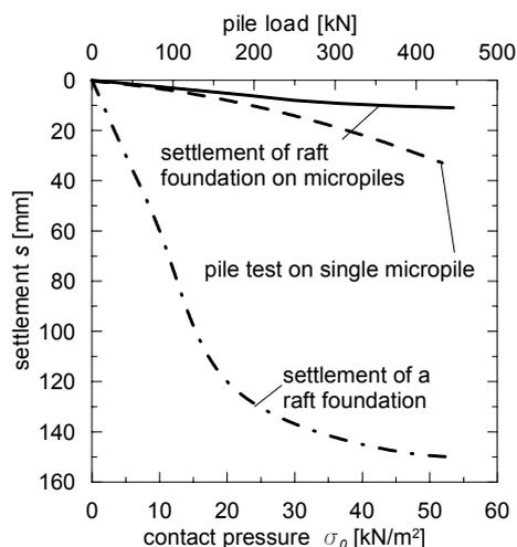
Figure 1. Settlement reduction effect of a raft foundation on floating micropiles (SSVP)
