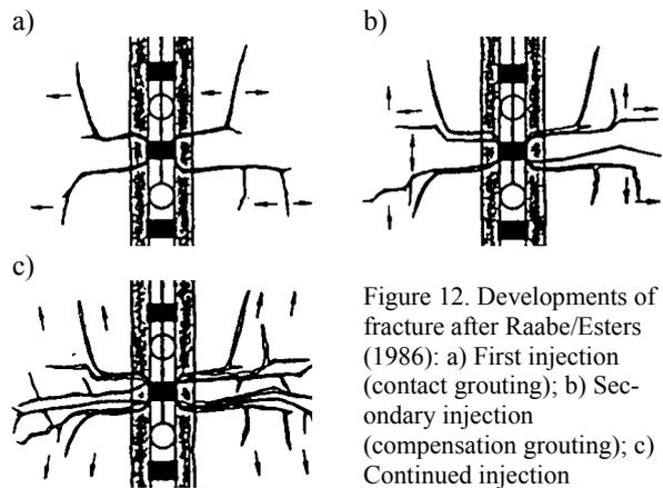
Figure 12. Developments of fracture after Raabe/Esters (1986): a) First injection (contact grouting); b) Secondary injection (compensation grouting); c) Continued injection
