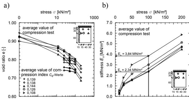
Figure 10. Stiffness of the model soil at different radial and vertical positions
