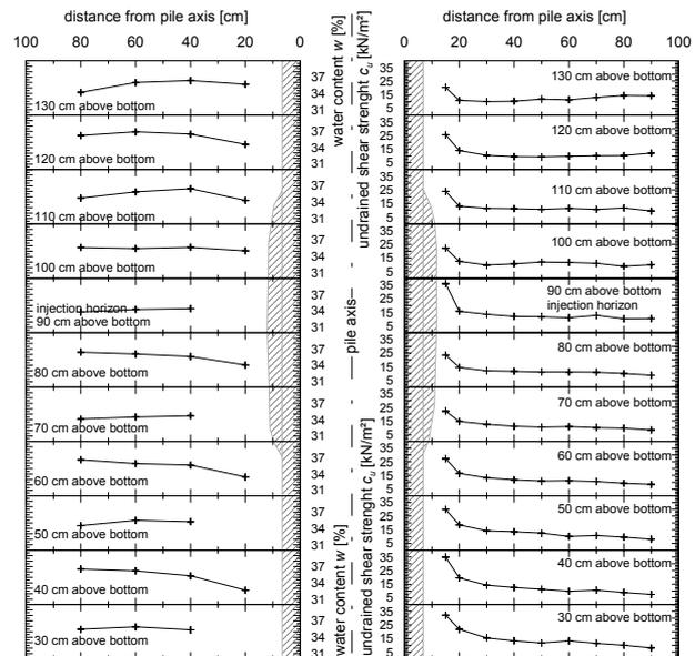
Figure 9. Water content and undrained shear strength
