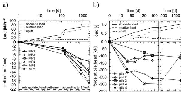
Figure 6. a) Settlement measurement and b) Measured force on pile head
