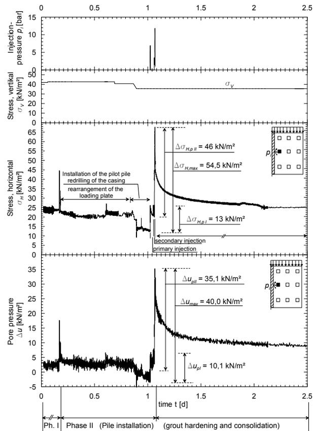
Figure 8. Example of test results: development of pore pressure and horizontal stress
