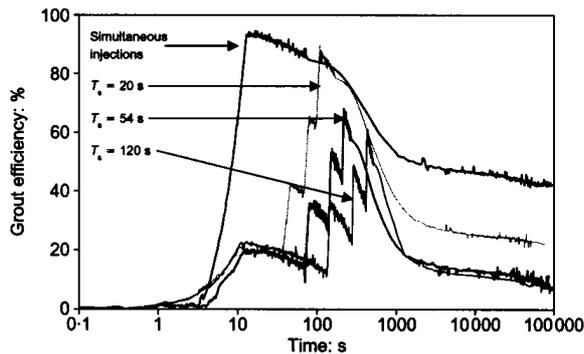
Figure 13. Grouting efficiency in normally consolidated soils (Soga et al. 2004)
