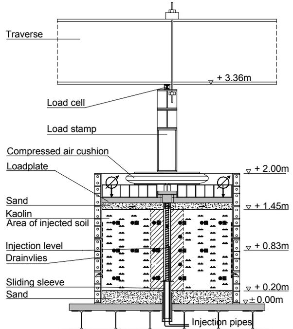
Figure 7. Model test on a segment of a micropile in soft soil
