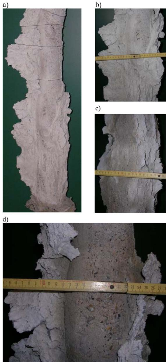
Figure 11. Exposed micropile showing the formation of vertical mortar sheet and expansion of the pile.
