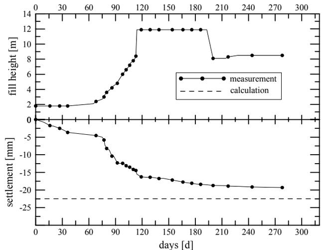
Figure 13. Settlements in a section with a concrete slab on top of the piles.
