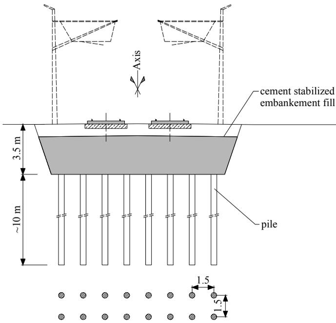
Figure 11. Cement stabilization in Beijing.
