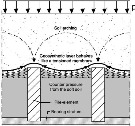
Figure 5. Mechanisms of load transfer and interaction.
