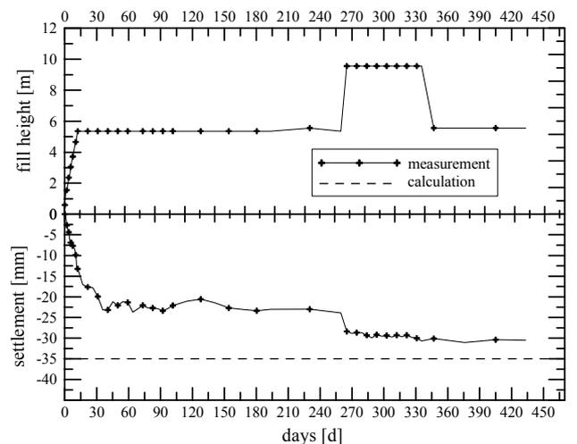
Figure 14. Settlements in a section with horizontal geogrid reinforcement on top of the piles.
