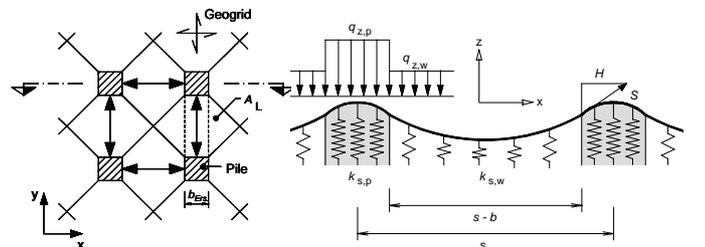
Figure 7. Loading of the reinforcement.
