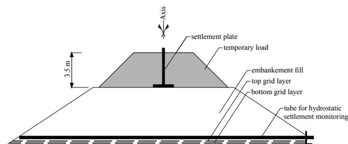
Figure 12. Typical measurement cross sections.
