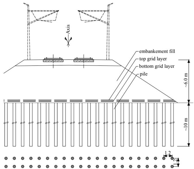
Figure 9. Geosynthetic-reinforced and pile-supported embankment Beijing.
