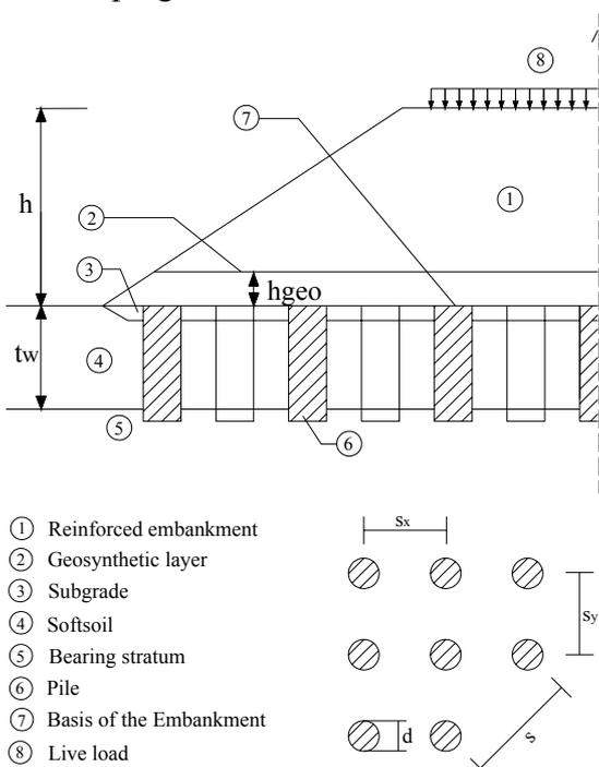
Figure 15. Geosynthetic-reinforced pile supported embankment (GPE) – Definition of parameters
