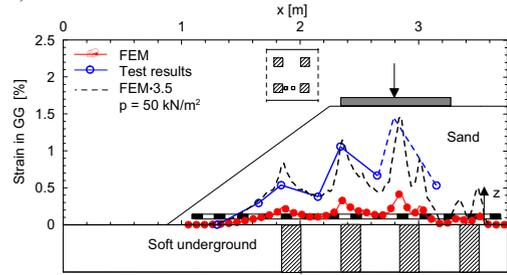
Figure 5. Strain in reinforcement (GG) a) unpiled and b) piled embankment
