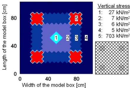
Figure 2. Vertical soil pressure distribution on the top of the geogrids, a) rectangular and, b) triangular pile arrangements
