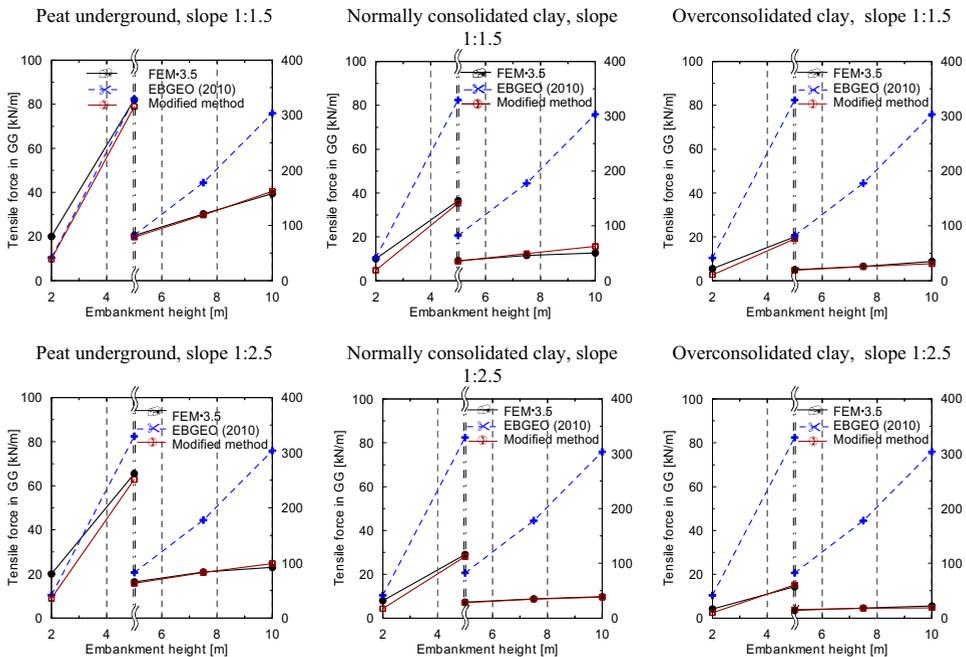
Figure 7. Comparison of tensile forces in reinforcement due to spreading according to the EB-GEO (2010) and the modified approaches at a surcharge pressure of  $p = 30$  kN/m<sup>2</sup>
