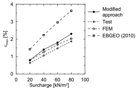
Figure 4. Comparison of strain in geogrids
