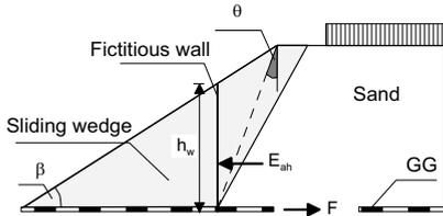
Figure 6. Sliding soil wedge
