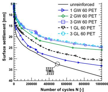
Figure 10. Surface settlement of the GEP-system
