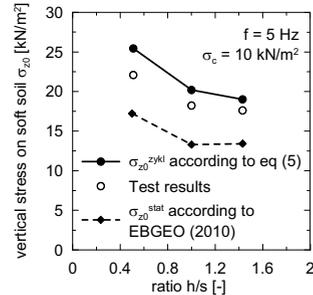
Figure 9. Comparison of equation (5) and model test results
