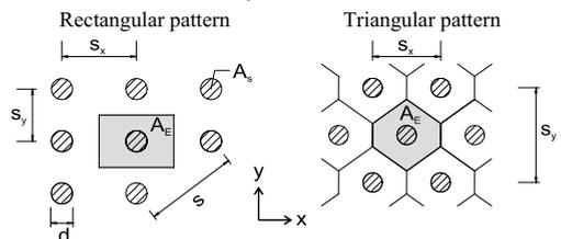
Figure 1. Arrangement of pile-like elements
