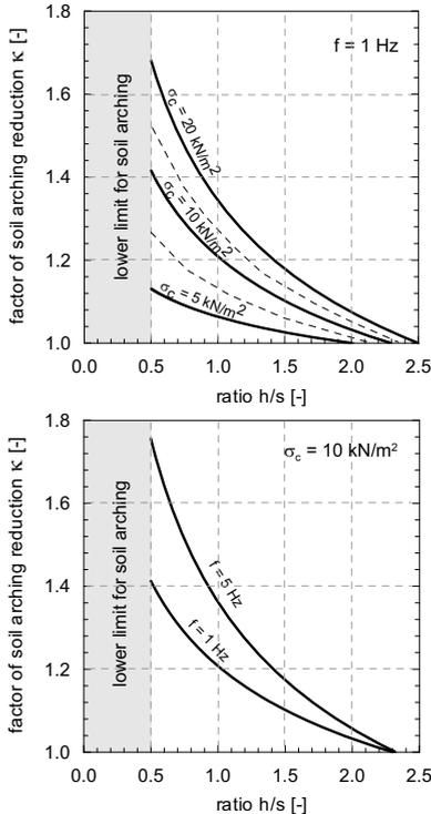
Figure 8. Soil arching reduction factor
