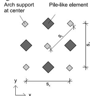
Figure 3. Modified spacing
