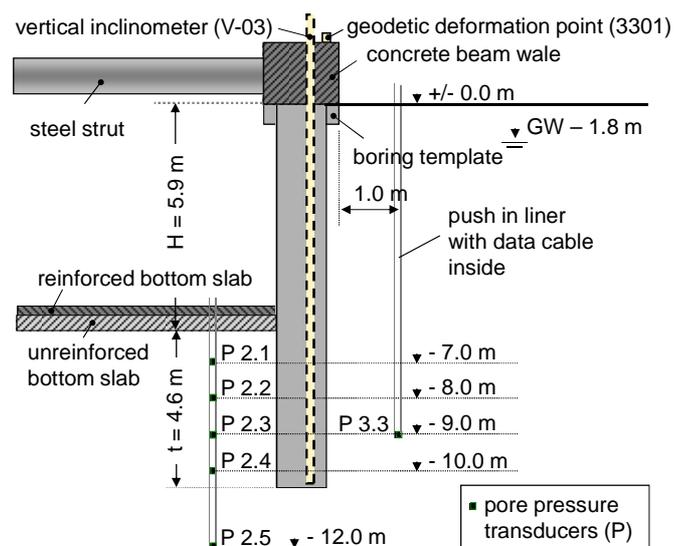
Figure 4. Monitoring section through bored pile wall showing pore pressure transducers, vertical inclinometer and geodetic deformation point
