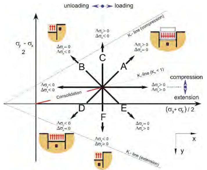
Figure 5. Idealized stress paths for triaxial tests
