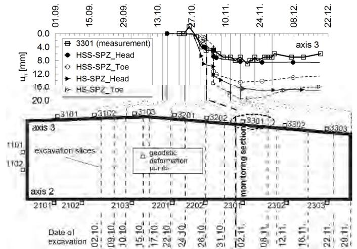
Figure 11. Comparison of calculated horizontal displacements at upper concrete beam wale with measurement results
