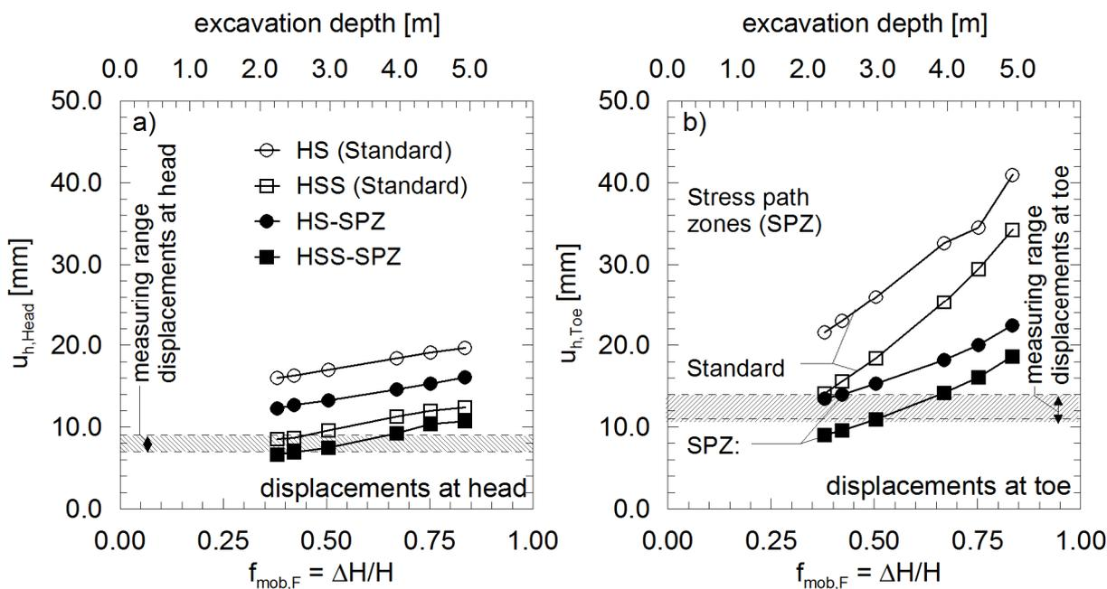
Figure 9. Influence of the mobilisation factor  $f_{mob,F}$  on horizontal displacements at the top (a) and the bottom (b) of the bored pile wall
