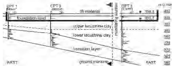
Figure 3. Underground condition in West-East cross section
