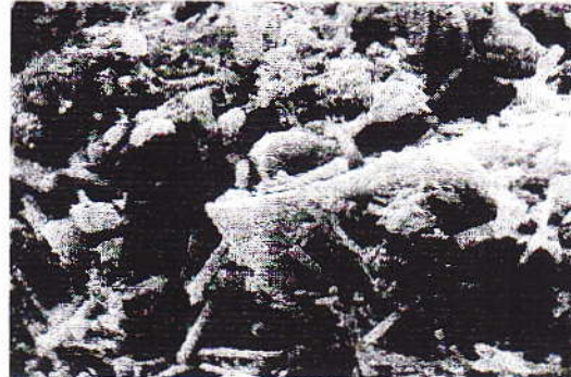
Figure 3. ettringite/portlandite at 180 days BB = 21 μm
