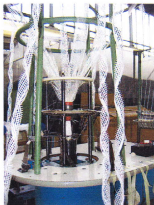
Figure 8: KEMAFIL® technology for manufacturing rope-like structures a) Processing unit b) Winding up a coil
