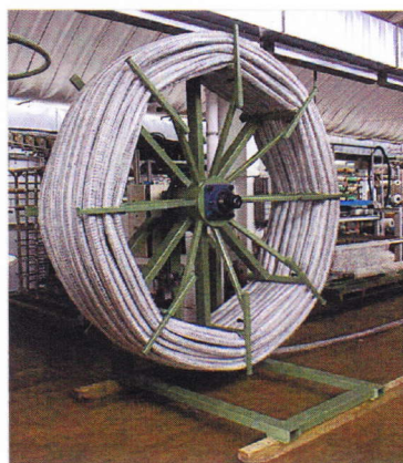
Figure 8: KEMAFIL® technology for manufacturing rope-like structures a) Processing unit b) Winding up a coil
