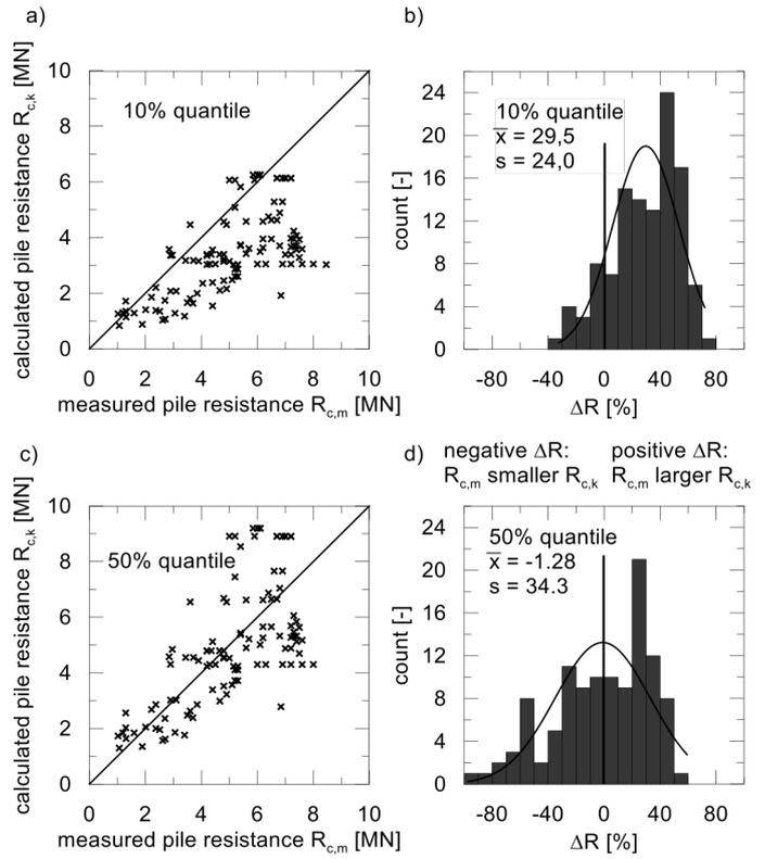
Figure 5. Results of the statistical calculation for the whole database of open-ended pipe piles for both quantiles; a) Scatter diagram (10 % quantile); b) Histogram (10 % quantile); c) Scatter diagram (50 % quantile); d) Histogram (50 % quantile)
