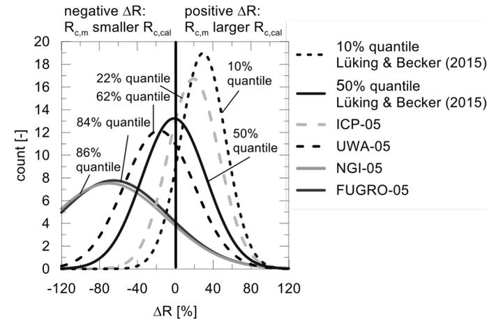
Figure 10. Histogram for different calculation methodologies after Becker & Lücking (2017) based on the database
