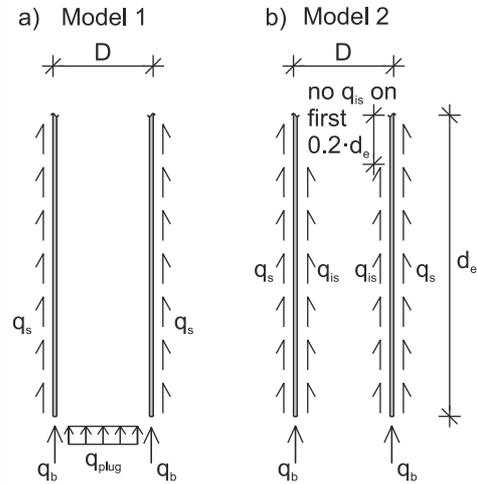
Figure 3. Calculation models for open-ended pipe piles, a) Model 1: Fully plugged condition, b) Model 2: No plugging
