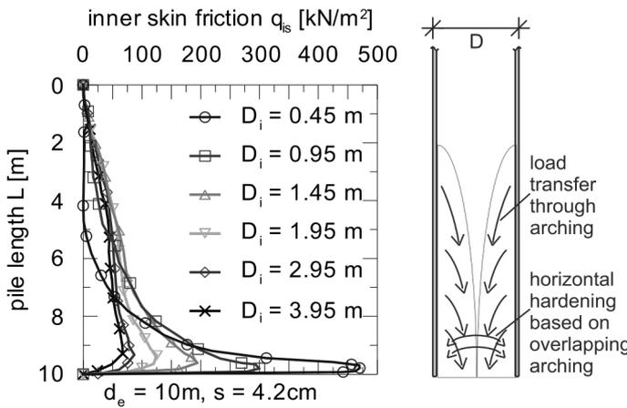
Figure 2. Inner skin friction for different pile diameter and model load transfer after Lüking (2010) and Lüking & Kempfert (2012)
