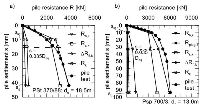
Figure 9. Comparison of a static pile testing with the calculations based on the values of experience (50 % quantile); a) H-piles; b) double H-piles
