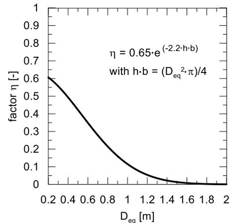
Figure 4. Factor  $\eta$  after equation (7) for considering the plugging effect for H-piles depending on the equivalent pile diameter  $D_{eq}$
