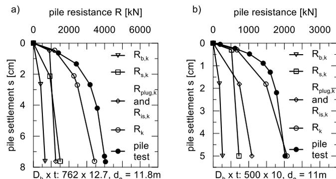
Figure 8. Comparison of a static pile testing with the calculations based on the values of experience (50% quantile)
