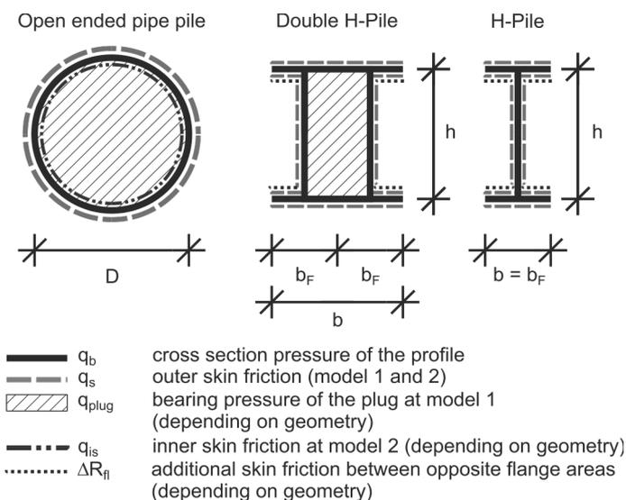
Figure 1. Profiles with different areas of possible plugging
