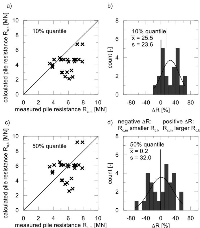
Figure 7. Results of the statistical calculation for the whole database of double H-piles for both quantiles; a) Scatter diagram (10 % quantile); b) Histogram (10 % quantile); c) Scatter diagram (50 % quantile); d) Histogram (50 % quantile)
