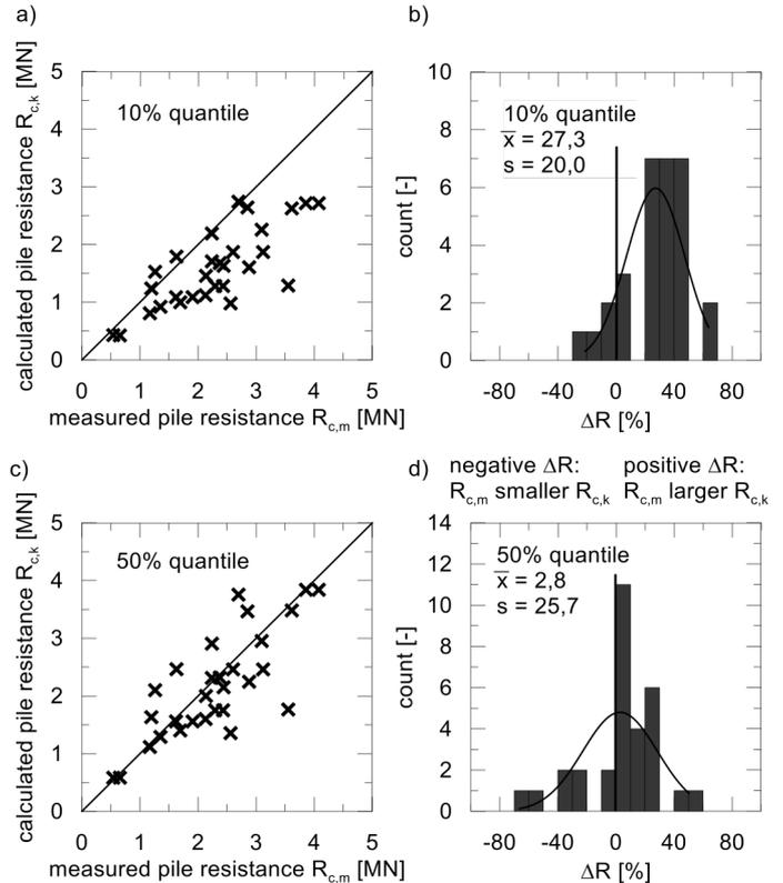
Figure 6. Results of the statistical calculation for the whole database of H-piles for both quantiles; a) Scatter diagram (10 % quantile); b) Histogram (10 % quantile); c) Scatter diagram (50 % quantile); d) Histogram (50 % quantile)
