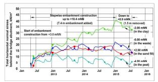
Figure 5. Total horizontal stresses  $\sigma_h$  at four levels and in four different layers behind the bridge abutment over time (see also Figure 3)
