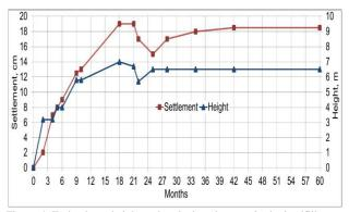
Figure 4. Embankmet height and typical settlements in the landfill area vs. time
