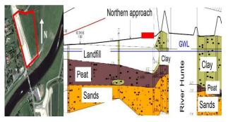
Figure 2. Landfill area below the Northern approach, left; typical geotechnical profile along the B212n, right
